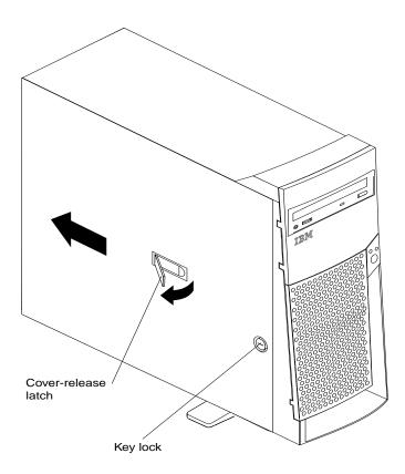
Complete the following steps to remove the side cover of the server:
